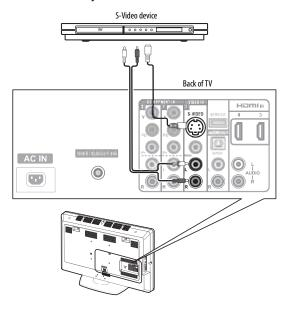
3 Connect an audio cable to the VIDEO IN 2 L and R audio jacks on the back of your TV and to the AUDIO OUT jack on the S-Video device.
